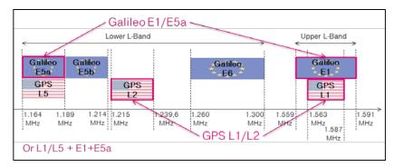
Delay at 1.5 GHz GNSS band (GPS L1 / Galileo E1) differs from delay at 1.2 GHz GNSS band (GPS L2 / Galileo E5
