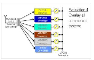
Multi-band systems are as expected between single-band and ePRTC (Cs + GNSS).
