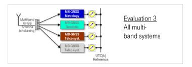
All multi-band systems fulfill PRTC-B masks for MTIE and TDEV <a>Some systems</a> are able to fulfill the stronger ePRTC mask
